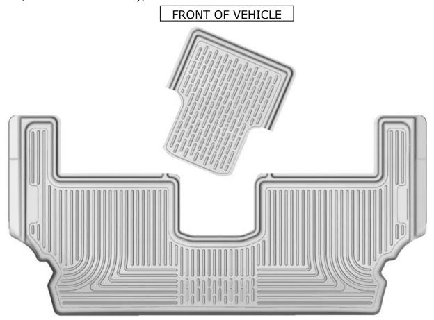
TO INSTALL YOUR LINER IN A PACIFICA WITH  $2^{ND}$  ROW BUCKET SEATS, FIRST SLIDE BOTH 2ND ROW SEATS FORWARD TO ALLOW EASIER ACCESS TO THE 3RD ROW FLOOR. WITH THE SEATS MOVED, INSTALL THE LINER POSITIONED AS SHOWN ABOVE. NOTE THAT THIS LINER ONLY WORKS WITH  $2^{ND}$  ROW STOW-N-GO SEATS. (OVER)
